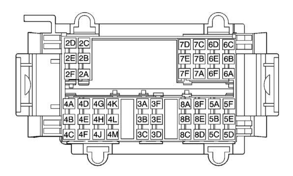
Fig. 39: Junction Block - I/P Bottom View Courtesy of GENERAL MOTORS CORP.
