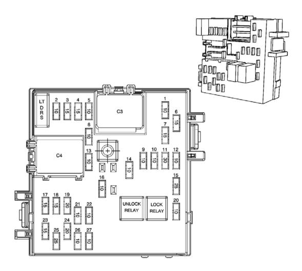
Fig. 33: Fuse Block - I/P Top View Courtesy of GENERAL MOTORS CORP.
