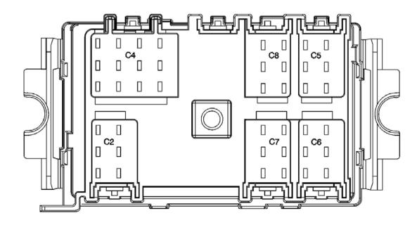
Fig. 38: Junction Block - I/P Top View
