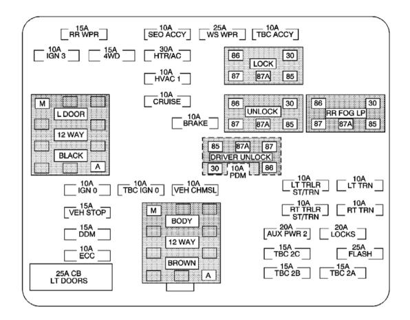
Fig. 32: Fuse Block - I/P Label Courtesy of GENERAL MOTORS CORP.
