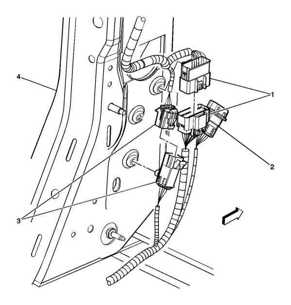
Fig. 18: Splice Pack SP207 Component Views Courtesy of GENERAL MOTORS CORP.
