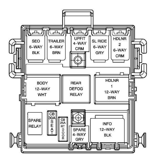
Fig. 35: Relay Block - I/P Label Courtesy of GENERAL MOTORS CORP.
