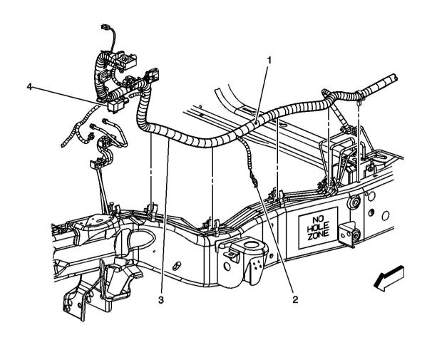
Fig. 8: Electronically Controlled Air Suspension Relay and G300 Component Views Courtesy of GENERAL MOTORS CORP.
