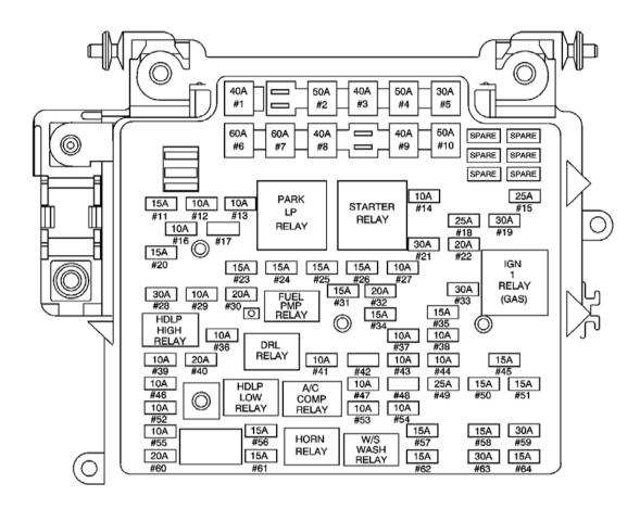
Fig. 30: Fuse Block - Underhood Top View Courtesy of GENERAL MOTORS CORP.
