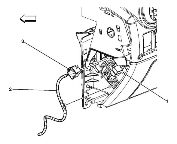
Fig. 2: Fuse Block - I/P Component Views Courtesy of GENERAL MOTORS CORP.
