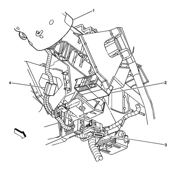
Fig. 17: Splice Pack SP206 Component Views Courtesy of GENERAL MOTORS CORP.
