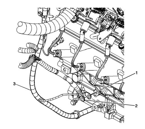
Fig. 12: G102 Component Views Courtesy of GENERAL MOTORS CORP.
