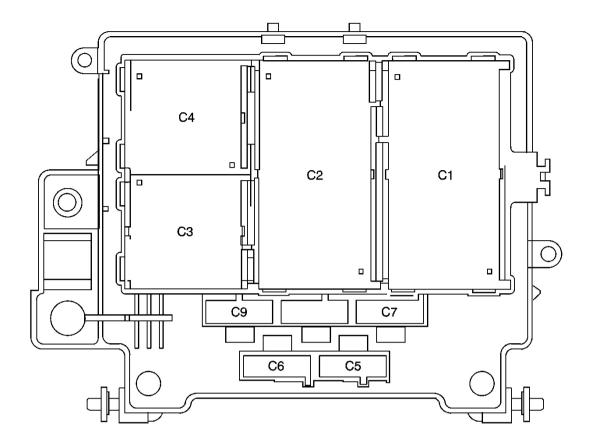
Fig. 31: Fuse Block - Underhood Bottom View Courtesy of GENERAL MOTORS CORP.
