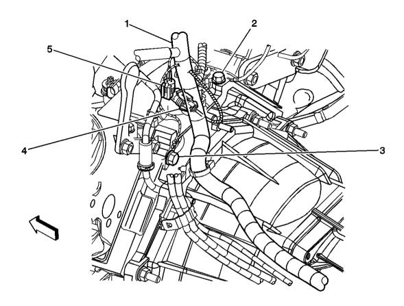
Fig. 11: G103 and G104 Component Views Courtesy of GENERAL MOTORS CORP.
