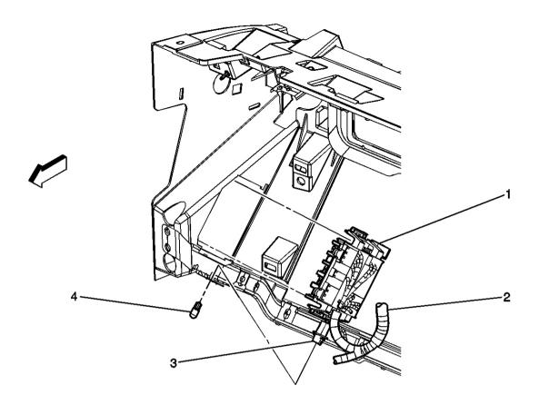
Fig. 4: Junction Block - I/P Component Views Courtesy of GENERAL MOTORS CORP.
