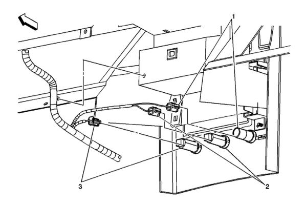
Fig. 5: Accessory Power Outlets - IP Component Views Courtesy of GENERAL MOTORS CORP.
