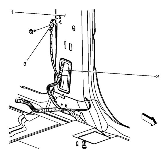
Fig. 20: G302 Component Views Courtesy of GENERAL MOTORS CORP.
