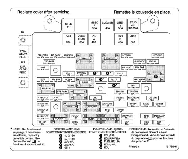
Fig. 29: Fuse Block - Underhood Label Courtesy of GENERAL MOTORS CORP.
