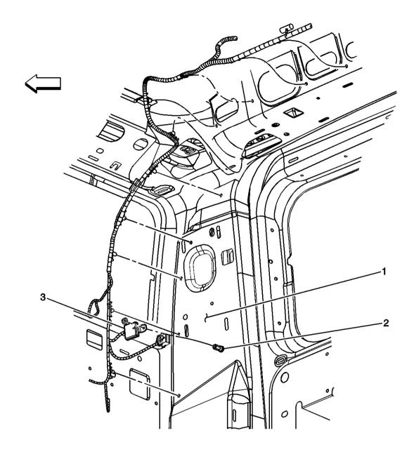
Fig. 27: G410 and SP410 Component Views Courtesy of GENERAL MOTORS CORP.
