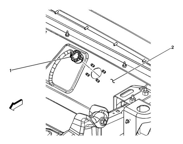
Fig. 28: Trailer Receptacle Component Views Courtesy of GENERAL MOTORS CORP.
