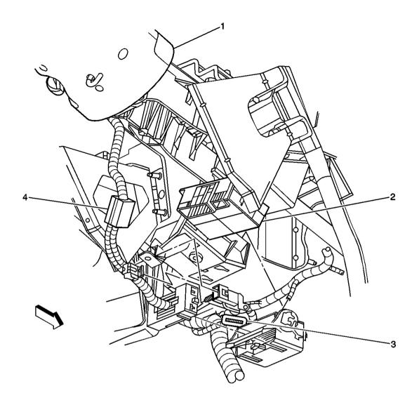
Fig. 9: Steering Wheel Controls Backlight Fuse Component Views Courtesy of GENERAL MOTORS CORP.
